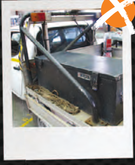
INSERT 18: No mesh window protection, black pipe structure bolted only to aluminium tray.
