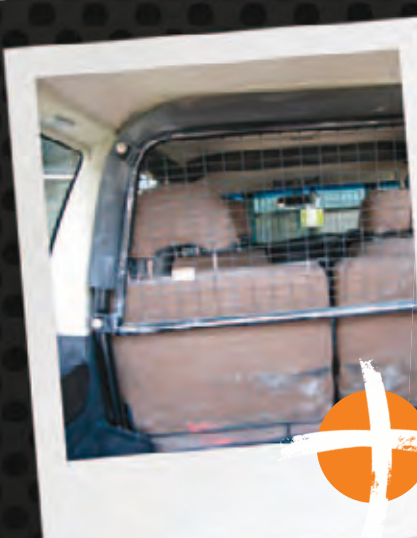
INSERT 10: Non load rated mesh, no rear bracing, no B or C pillar mounting.
