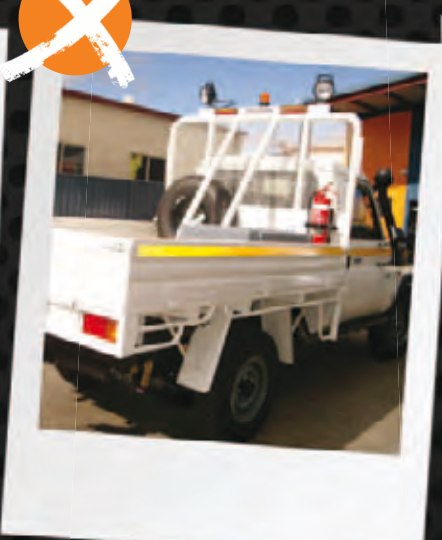
INSERT 23: ROPS is too high, and is only bolted to the tray pedestals.
