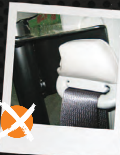
INSERT 4: B pillar mounting disables belt height adjustment with unpadded protrusion.
