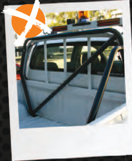
INSERT 17: External black pipe structure mounted in tub body only.
