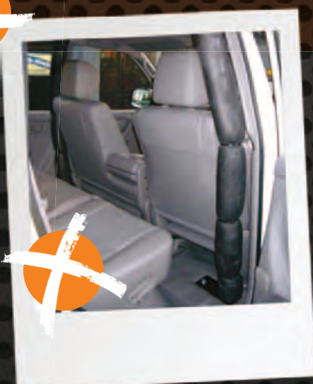
INSERT 15: Non compliant padding and single bolt floor mounting.
